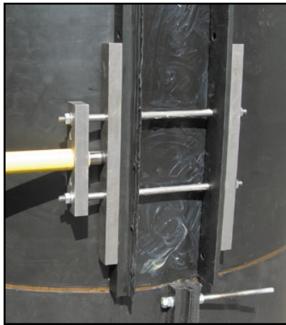
1. A new hydraulic clamp now rapidly pulls the jacket seams together.
