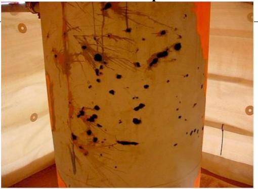
After removal of the clamps the full extent of the damage was evident. A total of 461 holes were found within a 15 metre section
